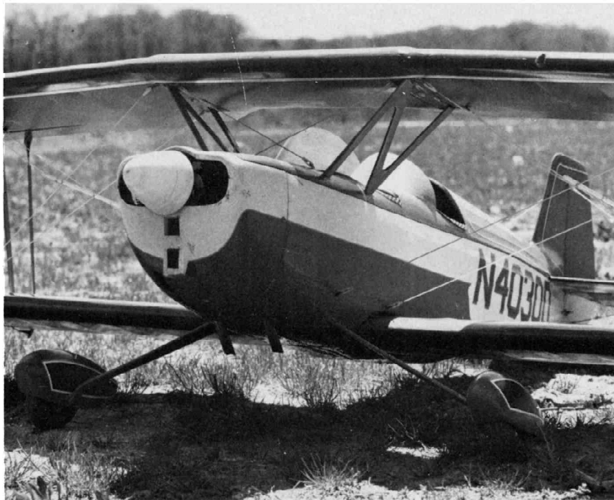
A side-mounted Fox 78 gives plenty of power for the NSPA aerobatic sequence. The engine is well-disguised in the cavernous cowl.
