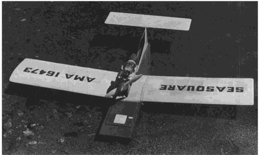
The pugnaous looking, square bow is easy to construct, leaves plenty of radio room, and protects the prop from power-killing water splashing. Hatch cover is rubber grommeted.
