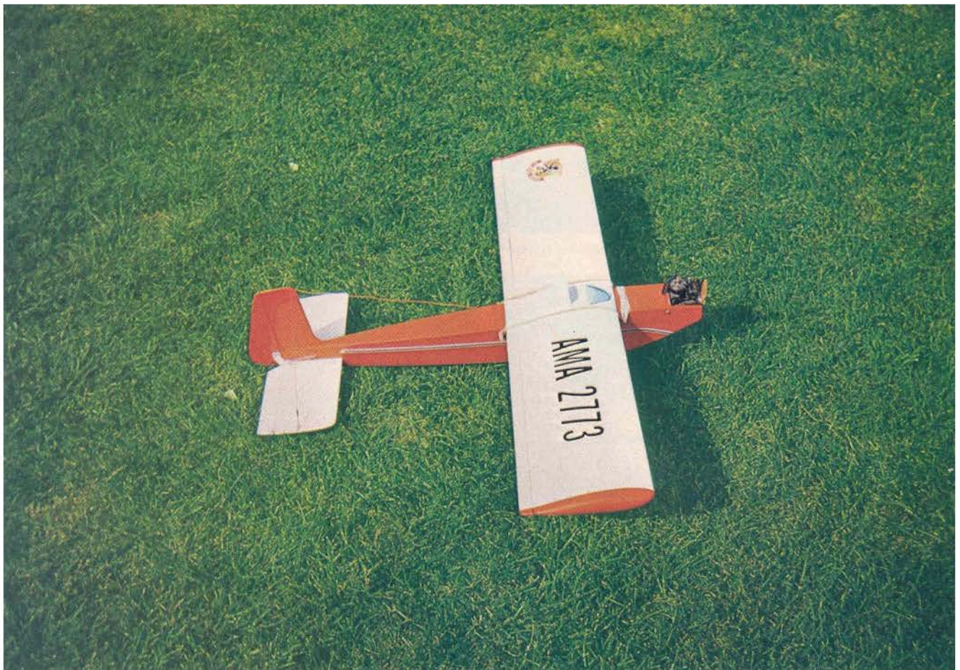
The 'Scotch Lass' with O.S. Max .15, E.K. Logictrol radio, and Super MonoKote covering. Wipe MonoKote with acetone before applying Finishing Touch decals.
