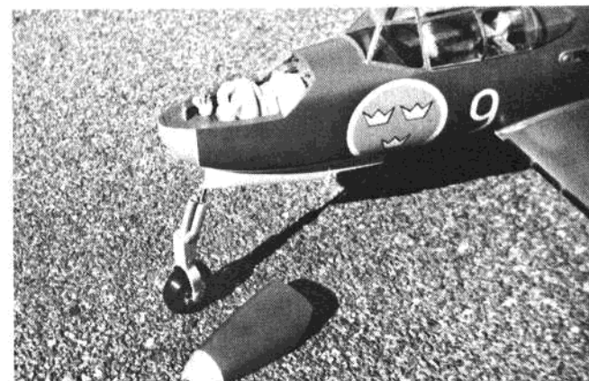
The access hatch to the battery compartment is molded from fiberglass.
