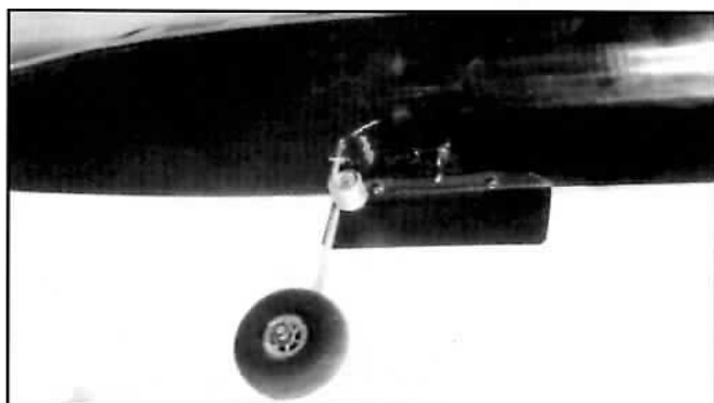
LEFT: A standard size servo activates both inboard and outboard elevons through a "Y" pushrod. RIGHT: Nose gear door bolted in place.
