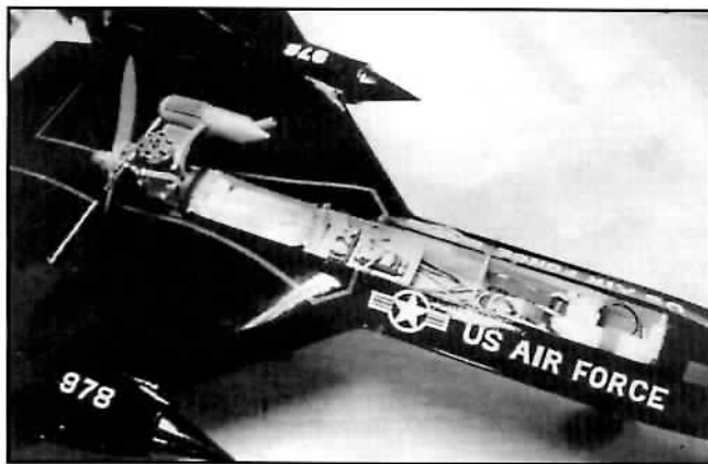
LEFT: Engine, prop, muffler, and fuel tank installed. RIGHT: Linkage for rudders and nose gear shown. Note the position of RX switch and charging jack.
