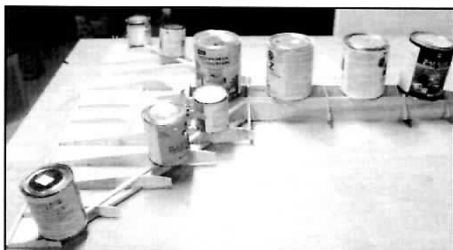
LEFT: Engine mount and firewall shown. The openings for fuel tube, throttle pushrod and hatch dowels were drilled later on this prototype (see text). Nose gear mount has been installed on W3. RIGHT: Construction of fuselage, make sure everything is built flat on building board.
