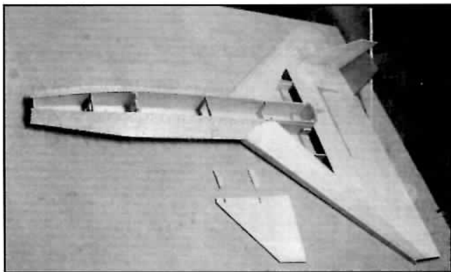
LEFT: Leading edges and fuselage longerons glued in place. When dry, add F3B. RIGHT: Add upper wing skins and fuselage side panels. Use template when gluing fins in place.
