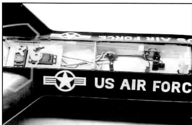
LEFT: Engine, prop, muffler, and fuel tank installed. RIGHT: Linkage for rudders and nose gear shown. Note the position of RX switch and charging jack.
