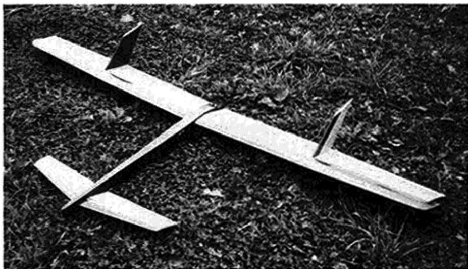
The vertical fins on the SC-3 each have a vertical spar which "plugs in" to a reinforced box structure. To align each fin, a small 1/16 inch dowel at the rear of the fin keeps it nice and straight.
