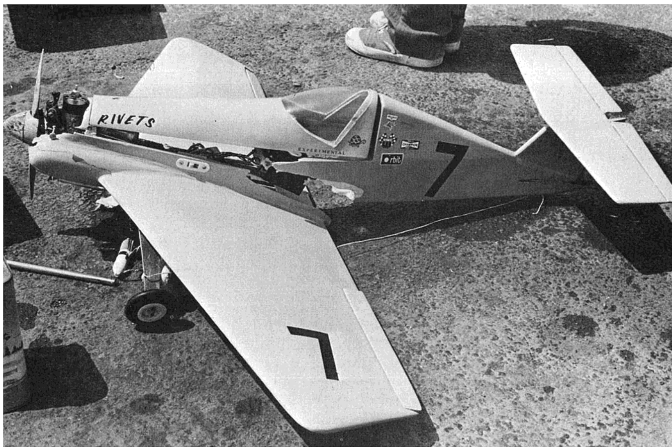
One of the photographs you usually never see in magazine construction articles! Photographed at L.A. Model Airport after Dick Sonheim decided to see what would happen if the C.G. was moved further aft.
