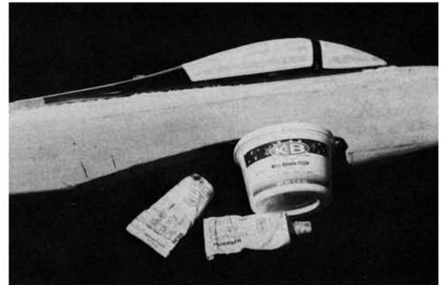
Canopy secured in place with cyanoacrylate adhesive and micro-balloons prior to making fillet.
