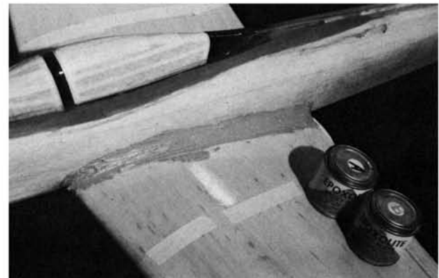
Wing fillets made from Sig Epoxolite.
