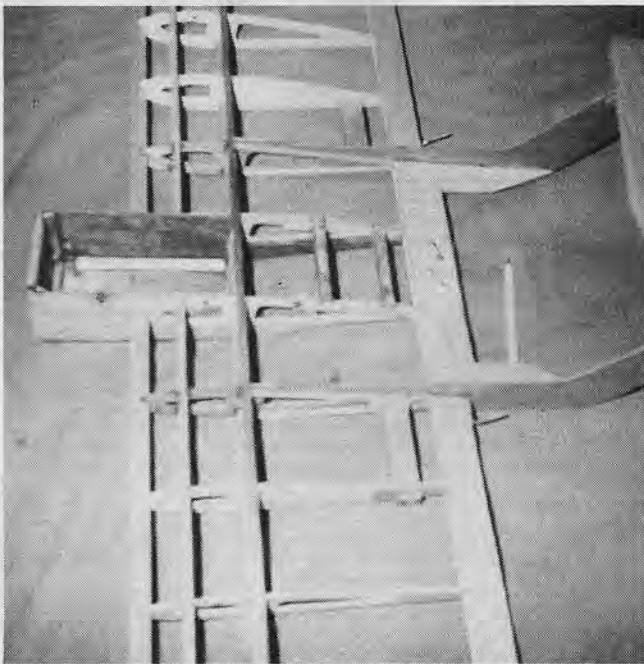
LEFT: Landing gear blocks, servo rails, and stab installed. RIGHT: Center section planked, radio boxes and servo trays ready for equipment.
