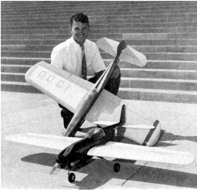
Author holds original 35-powered radio-controlled Nobler which was converted from control-line kit without refinements. It proved feasibility of developing design for contest performance.
