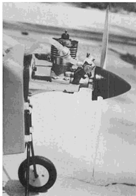
This side view clearly shows the downthrust wedge required to minimize stalling tendencies while under power.
