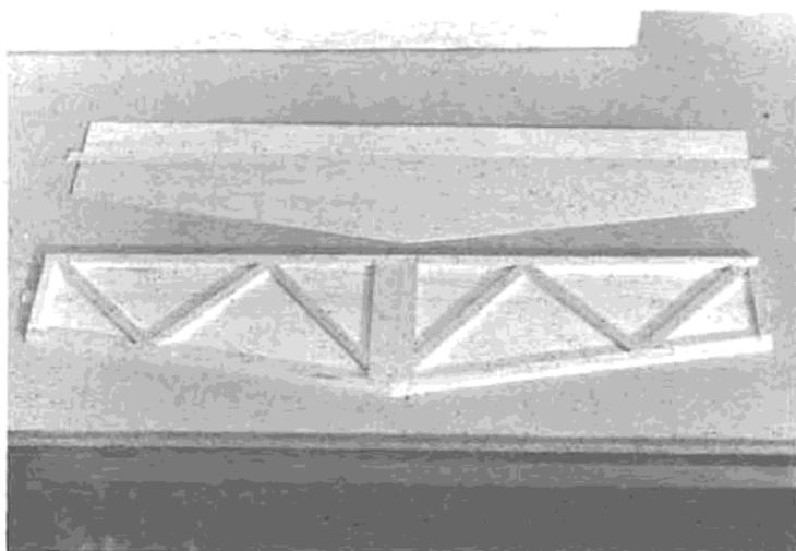
Glue all the internal stabilizer parts to the bottom stabilizer sheeting.
