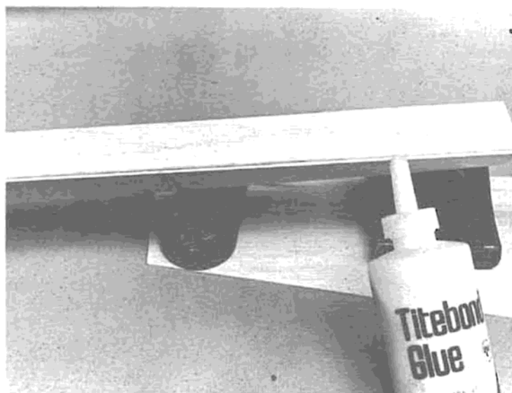
Bend the stabilizer sheets back on the masking tape and join together with a bead of Titebond glue, then weight down on a flat surface until dry.
