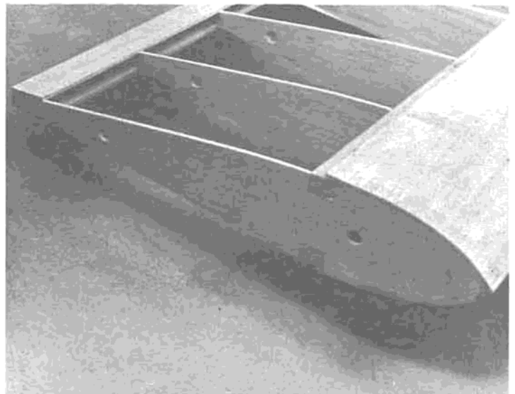
The wing panel is removed from the RCM Wing Jig and the ends sanded flush.
