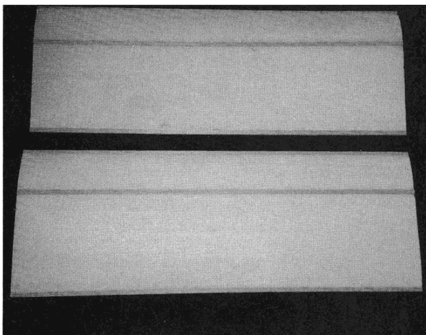
Wing cores with leading, trailing edges, and spars installed.
