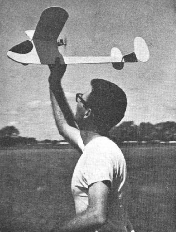
Designed for a slow steady climb, using a full tank of fuel to reach same height as a regular contest free flyer—Doc shows how to launch.
