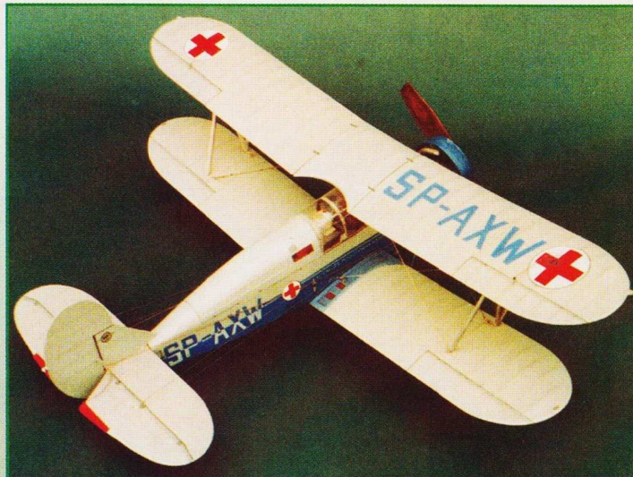
ABOVE LEFT: Loads of character. Bloodstained stretcher case. Exposed cable runs and control horns. Scale rib spacing using the 'sliced rib' technique detailed in plan. ABOVE RIGHT: The plans could be enlarged to suit larger C02 engines or used as a basis for a larger R/C or F/F version. 1/4 scale would be 9'4" and would make a great Glider Tug.
