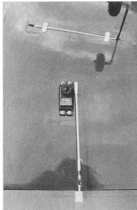
Detail of mounting elevon servo and pushrod on bottom side of wing. This set-up is possible when using electronic mixing, such as with Futaba 7UAF.
