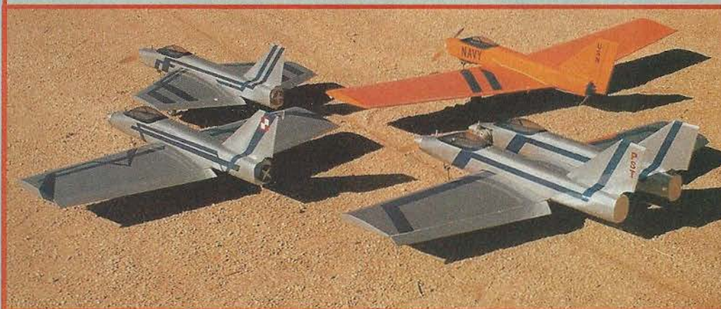
Teaser photo of Simitars to come. Left is Pole Star 40-60, next is Pole Star X (dubbed EPO, expert pilots only, by the Milwaukee Sqdn.), Pole Star Twin (pair of K&B 45's), and the Navy marked is the Pole Star FBI (Flies By Itself, it's 80" and flies like a free flight).
