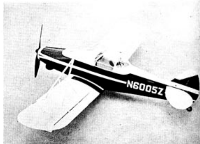
More scale points are shown in this photo—ailerons, flaps (workable), as well as landing and running lights and complete scale trim.
