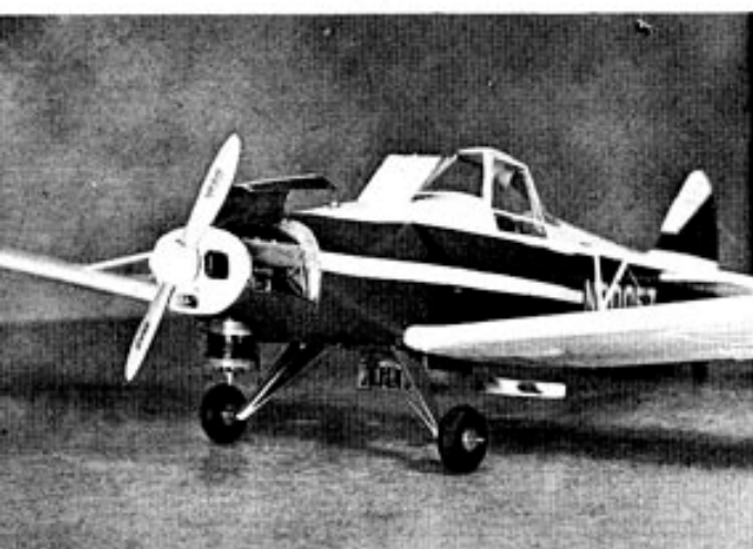
Most of the hatches are open in this photo—the dust bin hatch in front of the windshield and engine compartment hatches are open.
