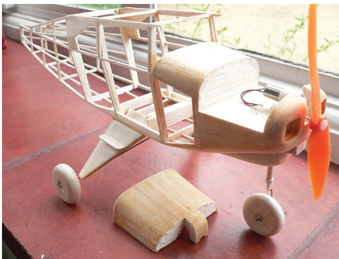
The basic fuselage after construction. Note the sheet in-fill between the stringers around the nose. You can also just see the way the rear upper side stringer joins rear of the window. The wheels are simple, having printed paper hubs for detail.
