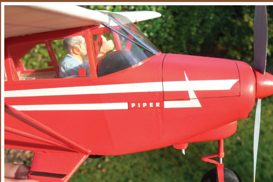
I printed the Piper logo on my laser printer. The paper panel was cut out and the white edges of the paper touched in with a red felt pen and glued in place with spray glue. This looks effective and the slight miss-match in the red tones does not notice once fixed in place.
