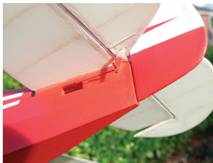
The control horns are made from 1/64" ply sheet. The end of the wire pushrod is simply held in place with sleeving cut from fine electrical wire, fixed with a tiny dot of cyano
