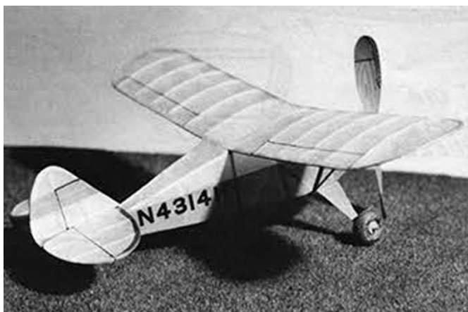
Generous flying surfaces make the Vagabond an excellent choice for Peanut scale. Note "grain" in the prop. Inked hinge lines nice touch.
