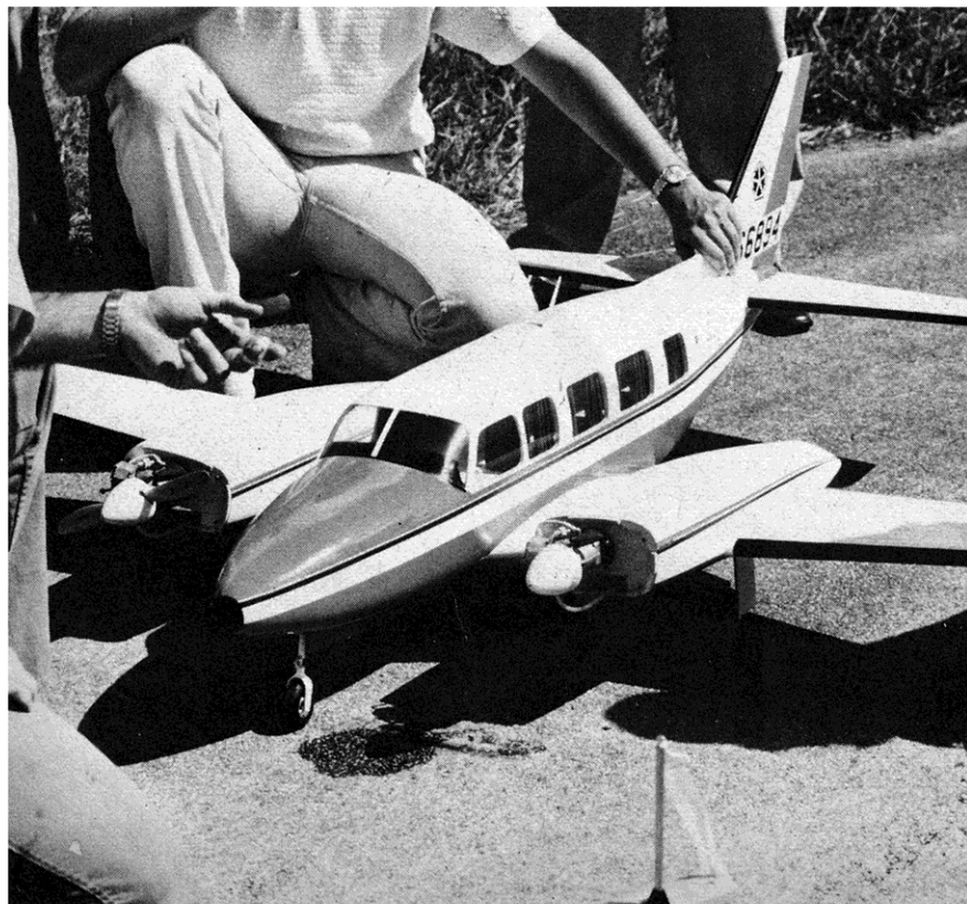
Engine tuning run-up sans cowlings prior to flight. Fiberglass cowlings are from one mold and are interchangeable. (Jay Miller photo)
