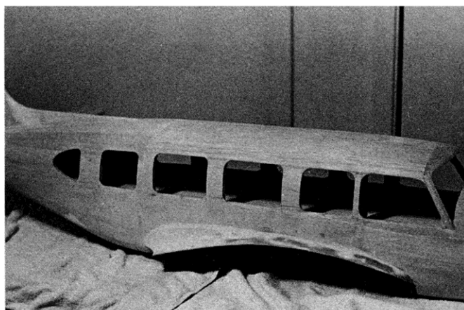
8 This photo shows the fuselage after being completely planked at the time the wing fillets are built up. Small balsa blocks and Sig Epoxolite accomplish the smooth fairing.
