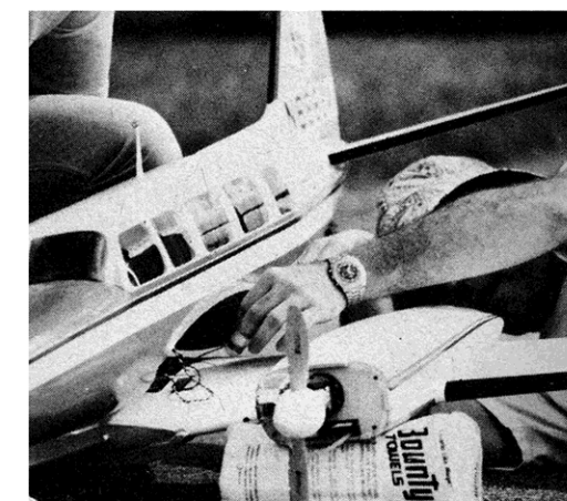
Builder/author Bugni is seen here making the necessary servo-receiver connections prior to fuselage-wing bolt down. (Jay Miller photo)
