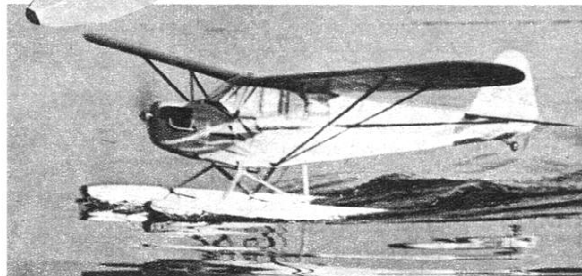
For plans of Chuck's J-3 Cub see the previous issue. Floats can also be used for free flight; can be scaled 40% of any wingspan.
