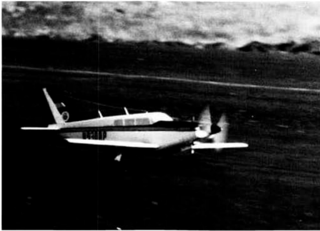
The Comanche just a split second before touchdown. Main wheels are almost on the deck, while nose gear is still high in proper fashion.
