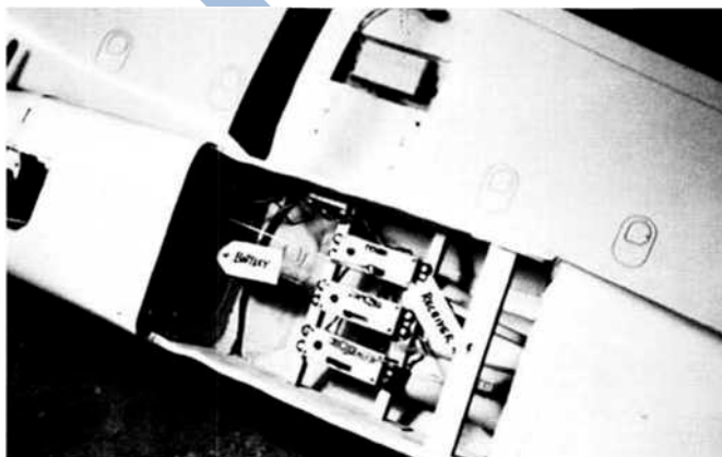
"In a canyon, in a cavern. . . Plenty of elbow room for radio installation here! Receiver is located behind servos.
