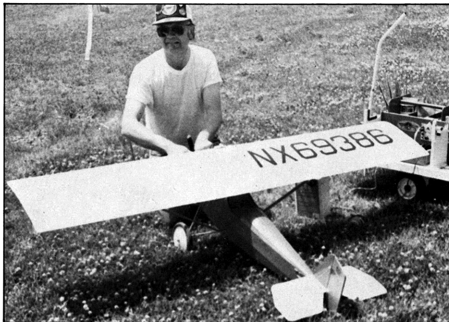
Author Tom Houle on the flight line with his 1/4 scale Pietenpol which should have very easy-flying characteristics, with its parasol wing and generous dihedral.
