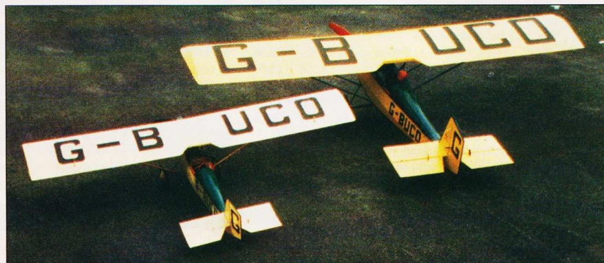
I was so impressed with the little Aircamper that I blew the plan up and produced a 68" version for i.c. power - both of the models are shown here.
