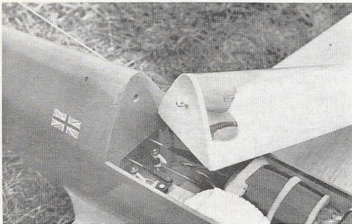
Radio and tank bay hatch is retained at rear by hardwood dowel which plugs into cockpit former. Front of hatch retained by a single bolt.
