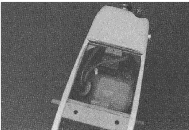
Fuel tank and nose steering installation.
