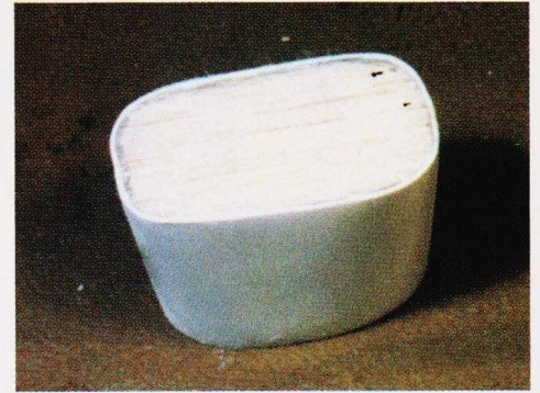
Fitting the tail cone with a bulkhead makes attachment easier and stronger.
