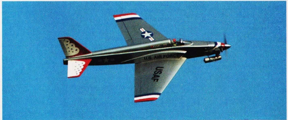
In flight, the SuperTigre G.61ABC pulled the plane like a rocket (above) though some initial plug problems caused erratic running. A Enya #3 plug made the problems go away. The nose gear was lengthened (below) about ½ inch to eliminate a negative angle of attack, that wouldn't allow rotation for takeoff.
