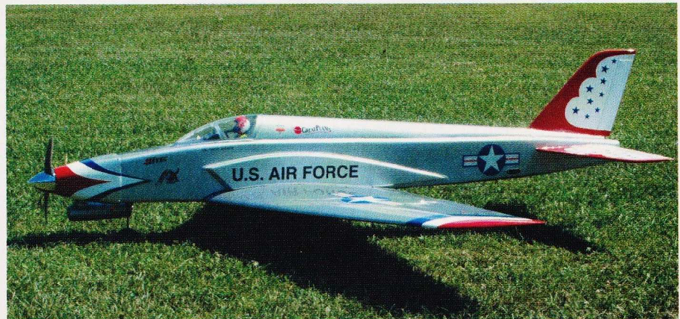
In flight, the SuperTigre G.61ABC pulled the plane like a rocket (above) though some initial plug problems caused erratic running. A Enya #3 plug made the problems go away. The nose gear was lengthened (below) about ½ inch to eliminate a negative angle of attack, that wouldn't allow rotation for takeoff.
