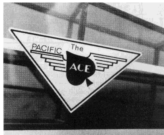
Pacific Ace logo close-up The material and lettering were not fuelproof and were destroyed on the left side by cleaner. Good decals are being considered.
