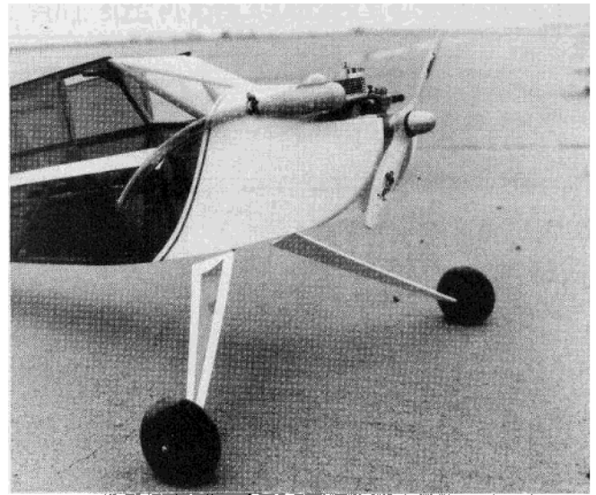
3/4 front view showing the O.S. .25 FSR with muffler and oil goo remover. Three inch Trexler wheels.
