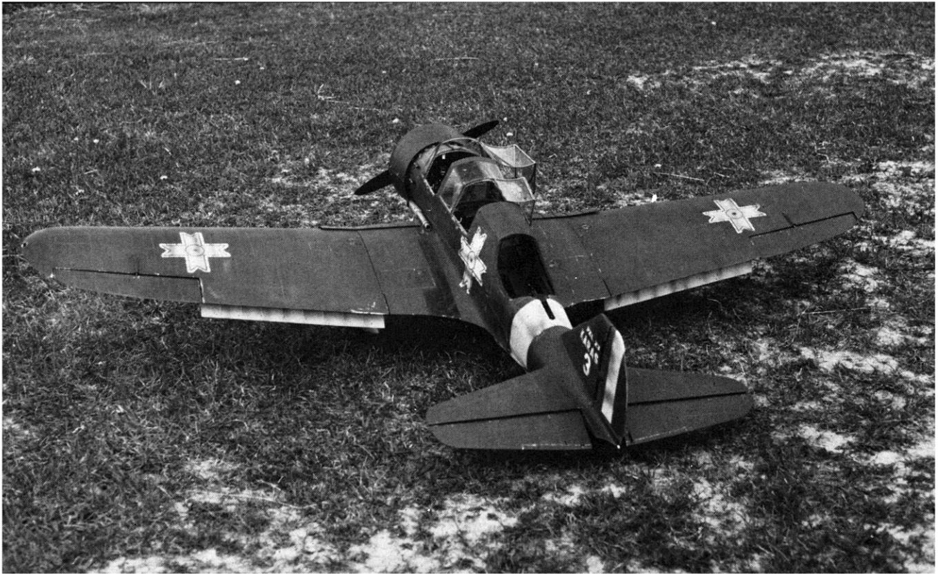
Functional canopies and split flaps are just two of the many operational features of the Karas.
