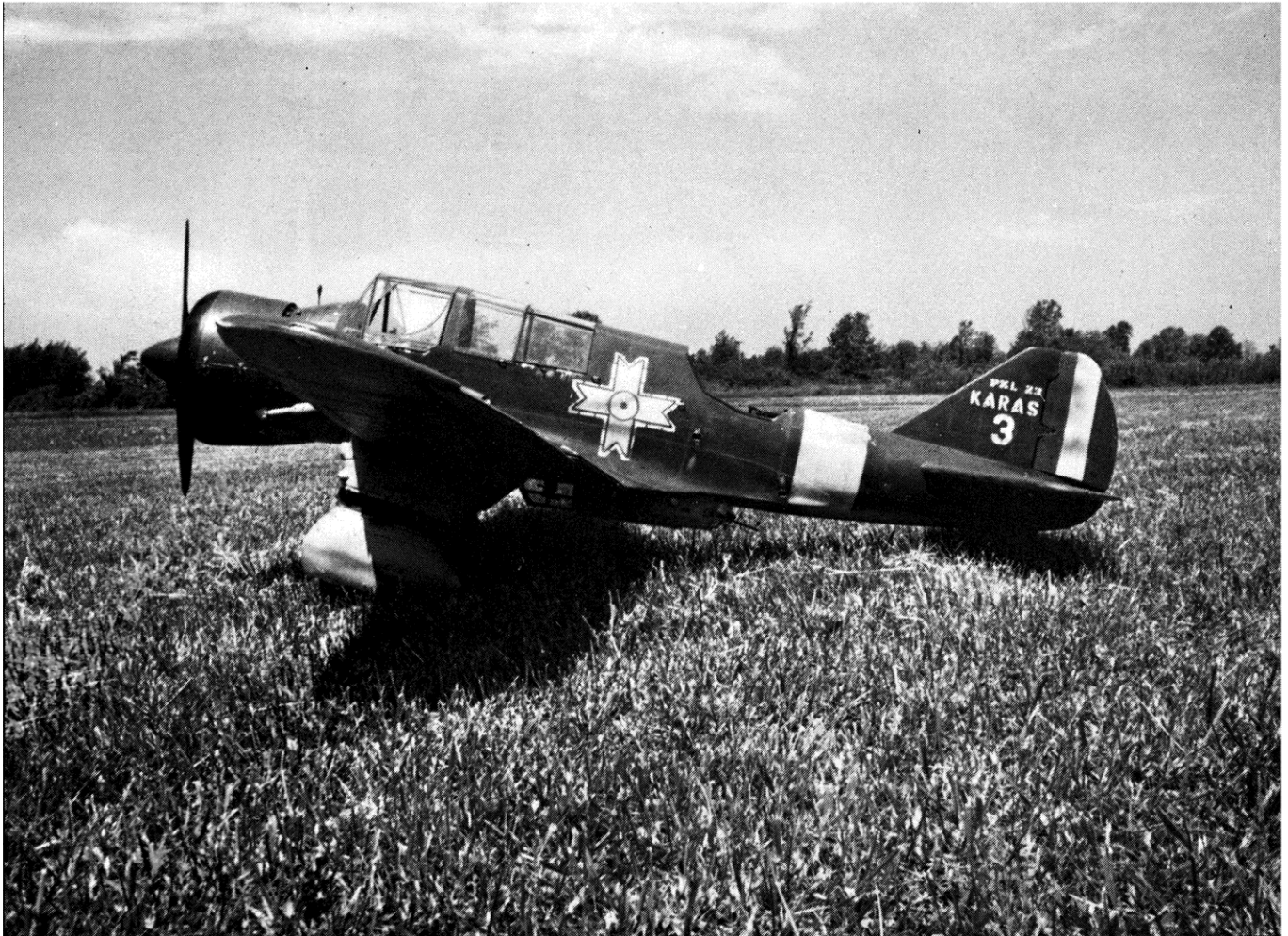
The Karas is a large model, spanning 99 inches, yet the wing loading is only 32 ounces-per-square-foot.
