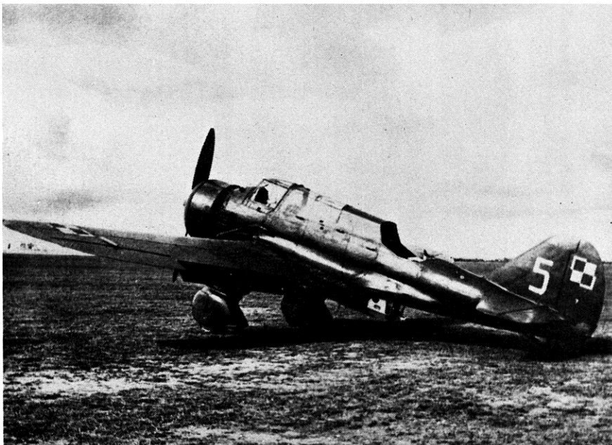
The all-metal P-23 carried a crew of three. (Photo courtesy L. Gordon)
