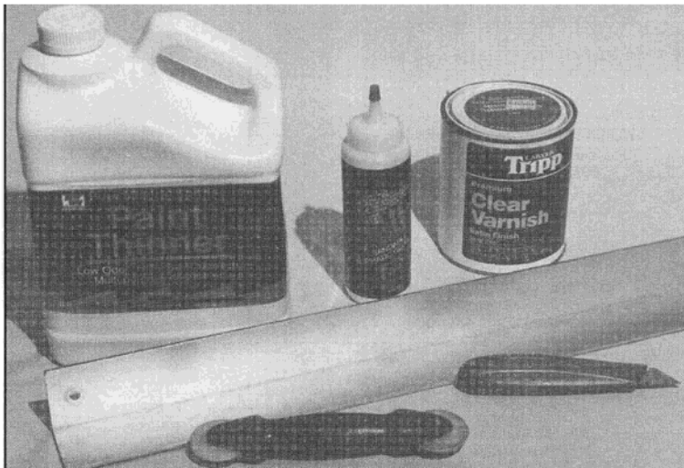
Some of the specialized materials and tools used in this project: paint thinner, aliphatic resin glue, polyurethane varnish, a long solid straightedge, a screen door rolling pin, and a utility knife.
