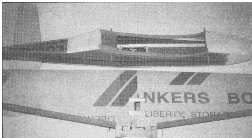
The completed airframe components ready for covering or painting. If you elect to cover with MonoKote, you can cut holes in the wing behind the spar, this will save 6-8 oz.
