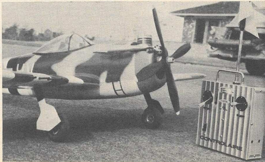
Fuselage is planked, time consuming, but easy to do. Controlaire R/C equipment.
