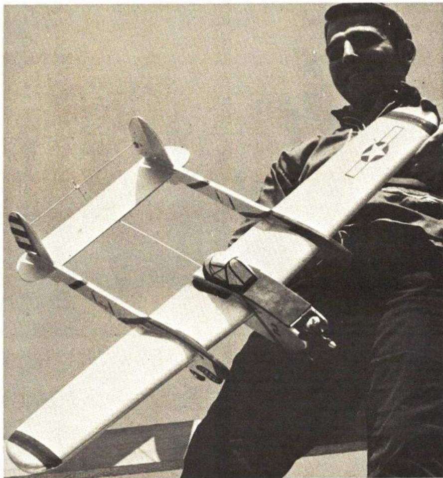
Foam wings, boxy fuse, and profile booms make it a snap. Note interesting linkage.
