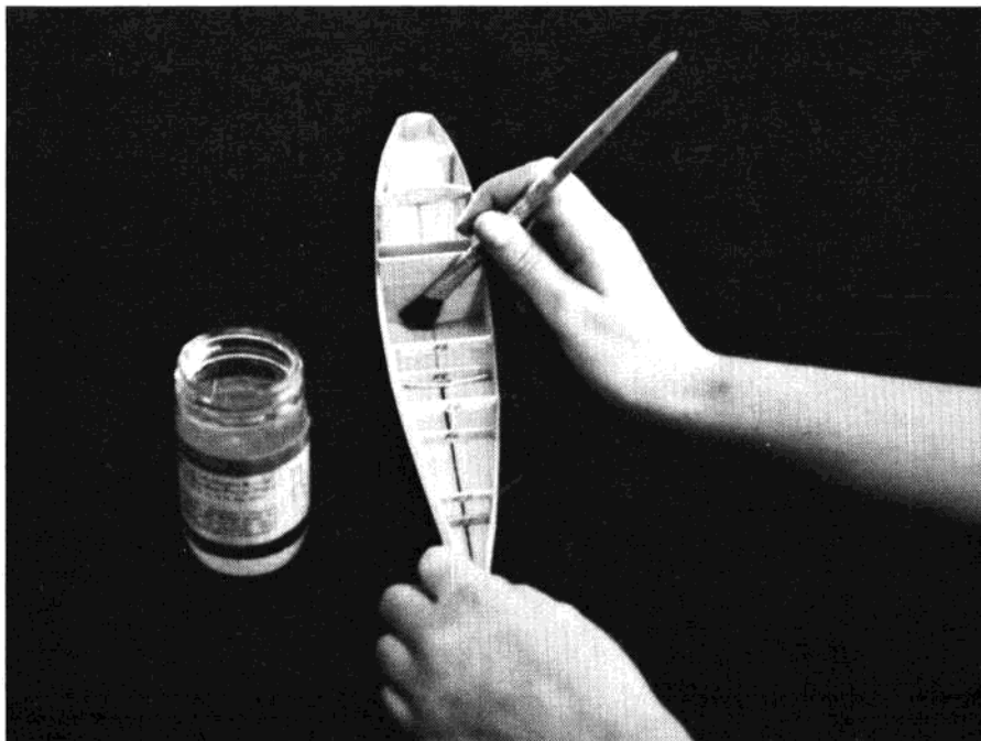
When hull is completed to this stage, apply two coats of thin clear dope to interior for waterproofing.
