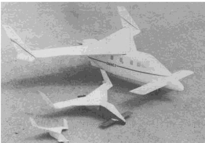
A family of Omacs. The 12-inch glider and 24-inch .020 F/F were built to prove the design's airworthiness before starting on the big one.
