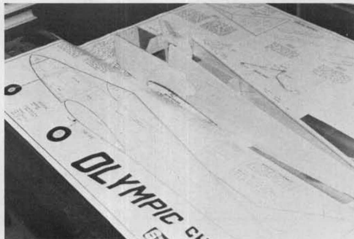
Fuselage construction is simple and basic. Note keved splice and overlapping ply and balsa doubler.
