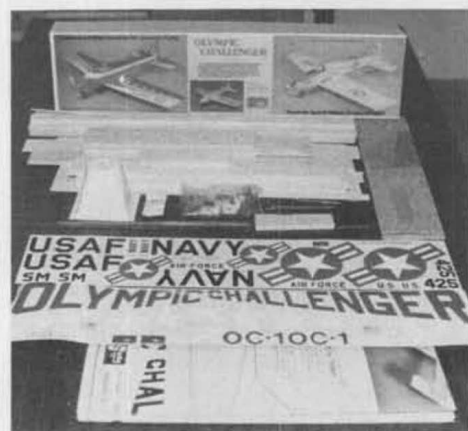
Out of the box. Die-cut parts, hardware, cowl, decals, strip and sheet wood, plans.
