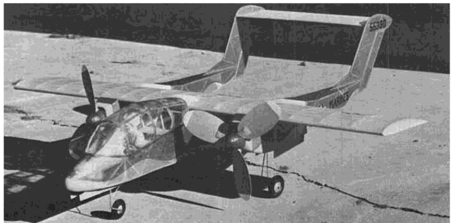
The Bronco has an efficient, powerful, mean look about it. Absence of dihedral may raise some eyebrows, but with counterrotating props and a low CG, roll stability is no problem.
