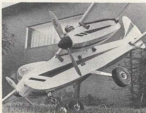
Close-up view of the underneath section shows simplicity of design, and bolted landing gear.
