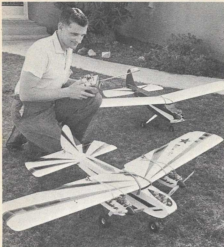
Author at the reed transmitter of his twin-engine machine. Original Nova is seen in background. Rubber-bands hold engine nacelles to wing.
