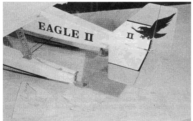
Tail group Eagle II template requires sharp #11 X-Acto blade. Spray tail with Windex, float on trim, slice at hinge line. Don't forget to seal edges with polyurethane.
