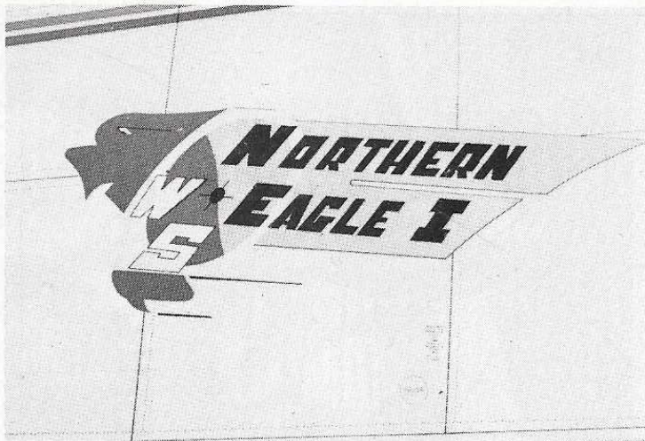
Finish is a delicately handled lace paint job on both the wing and stab. Also notice the anhedral stabilizer design. It's an exotic bird to see. At left: A paper mask technique and india ink produced unique insignia.
