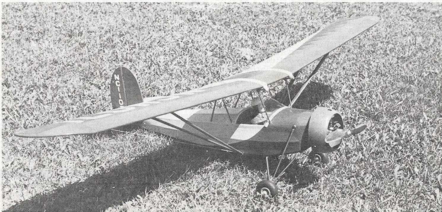
Author shows underside of prototype (above). Landing gear fabricated from music wire. Cowl for Nicholas Beasley comes from plastic soft drink bottle (below). Plane is typical of early light aircraft. It's cute.
