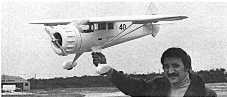
Noted FLYING MODELS author Nick Zirola was on hand to demonstrate his skill for first flights with the Mr. Mulligan (below). The ship flew well with no bad habits. It's stable and suitable for flyers with some background experience. It has high drag with that wide body and struts but that presents no problem.
