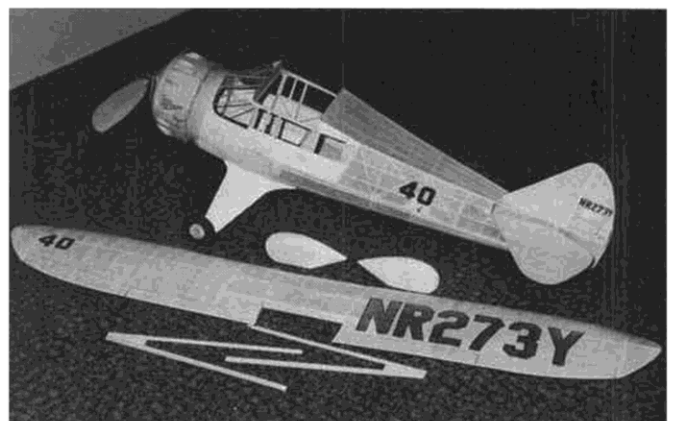
Though ship is quite stable in flight, Tom suggests that an extra half inch of dihedral per tip might make it even better.
