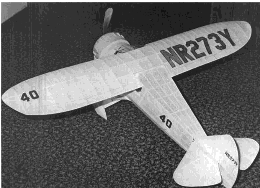
Phil Bernhardt revised Tom's drawings to show the scale wing tips, which tapered upward from the bottom. In effect, this added some tip dihedral. Scale stab offered no stability problems.
