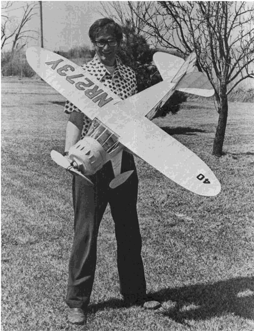
No, Tom is not a midget, that Mulligan has a 56 inch wingspan! Ship was designed directly over Hal Osborne's 1-3/4 inch-to-the-foot scale drawings (March/April '72 MB).
