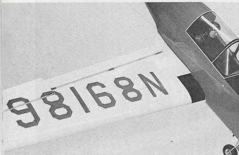
Stan hinged the flaps along the lower edge, feels it to be an advantage. Increased rate of sink helps over tree lines into marginal sized fields.
