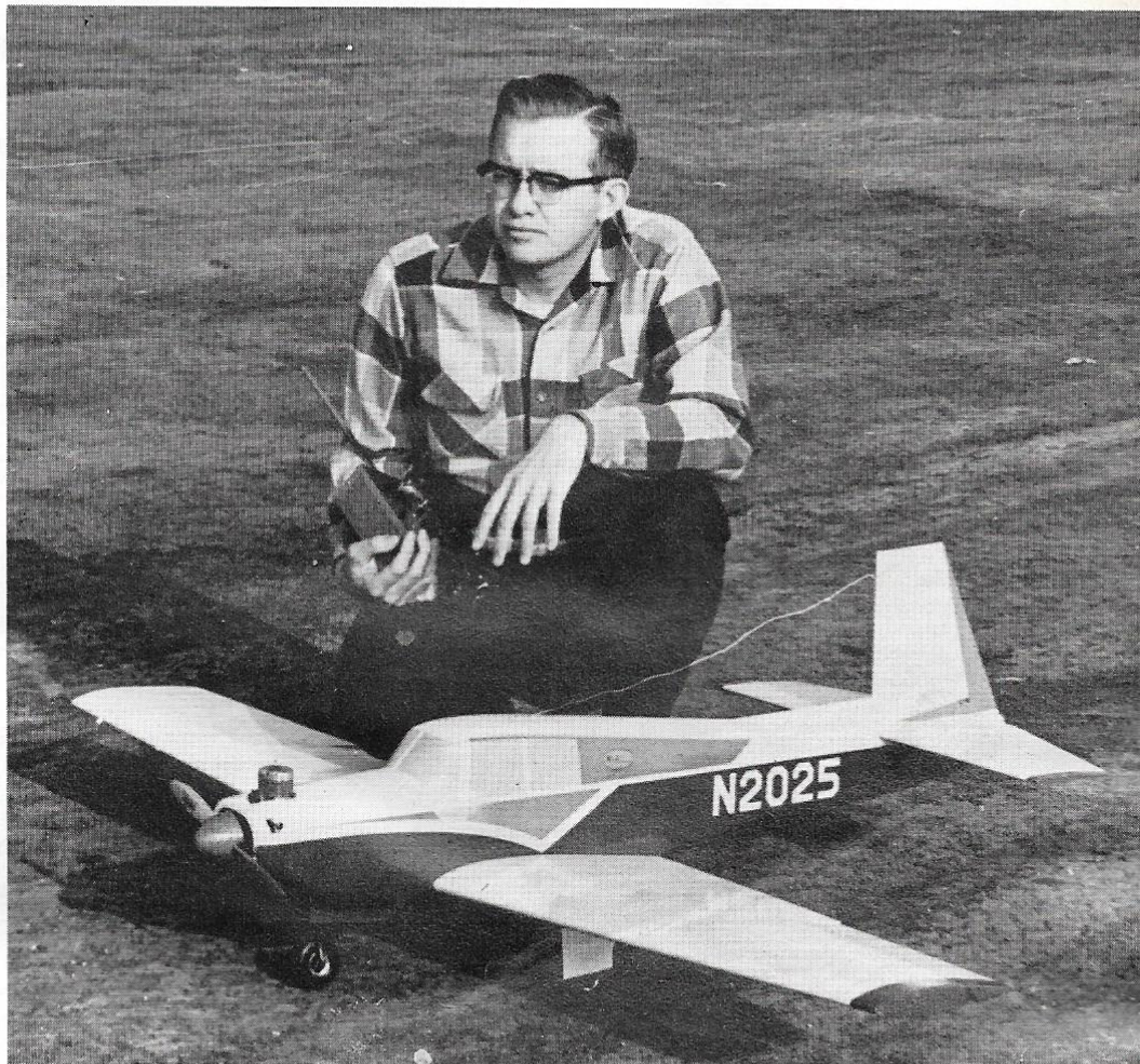
To keep light wing loading for aerobatics, the sharply tapered wings have long span. Airfoil is fully symmetrical which minimizes attitude changes with power variations.
