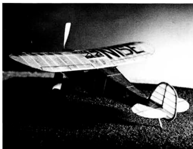
Long tail moment gives the little ship plenty of stability. Prop clearance is a little doubtful, but plastic is tough!
