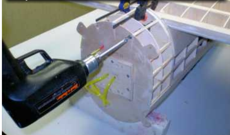
With the partially sheeted wing center section in place, drill holes in the leading edge of the wing for the wing dowels with a long drill. Holes in the formers guide the drill bit. Then remove the wing and glue two dowels in the wing. Note the removable firewall and cowl mounting tabs.
