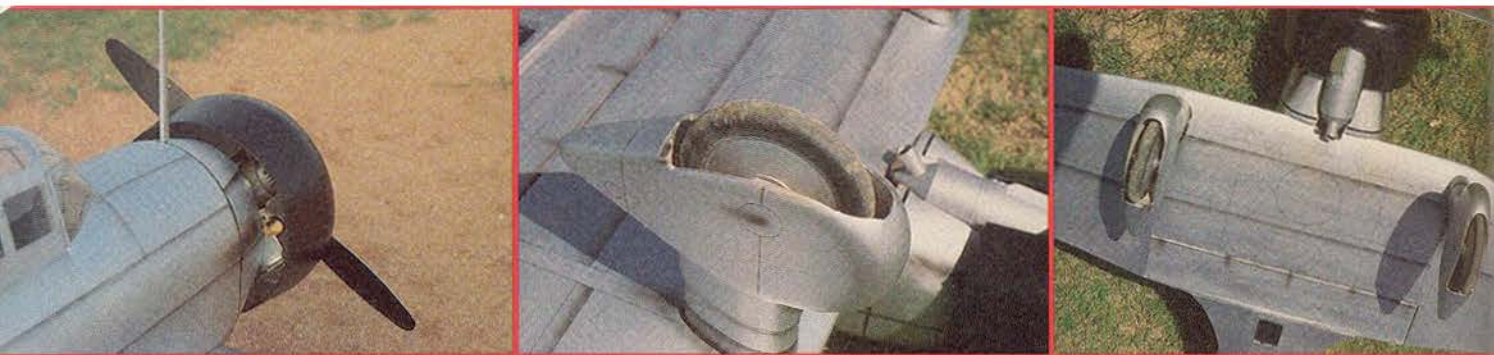
LEFT: Plywood and balsa cowl ducts airflow overhead of O.S. 91 FSR engine. Radio mast is removeable. Forward visibility was a hazard for Japanese pilots --- no problem for RC model. MIDDLE: Plenty of wheel clearance for Williams Bros. wheel in all-wood pant is requirement for good grass-field operation. Note clearance in wing surface for flex of coil-spring landing gear. RIGHT: Wide-stance landing gear yields good ground handling. Radio switch, jack and wing bolts are inside flap opening. Muffler is partially exposed. Observer's window aft of wing. Wheels have 1 degree toe-in each.
