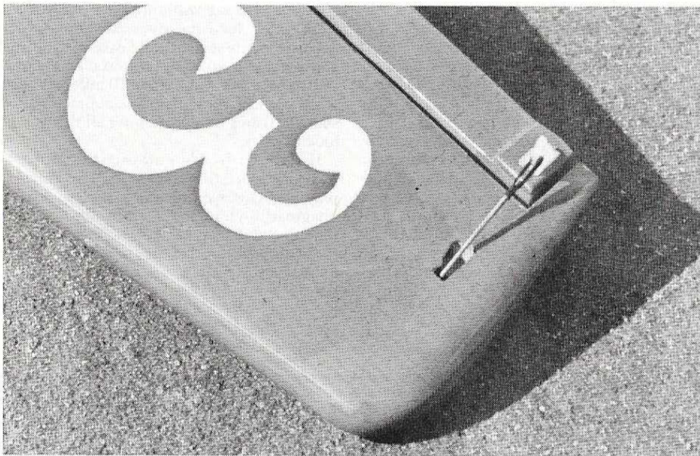
Aileron hook-up at each wing tip. This is a standard feature of Dan Reiss designs. Works well with foam wings. Top: Tail assembly details. Royal Products metal tailwheel bracket is the most durable for heavy models. At bottom: Detail of the wheel pants and Hallco gear. Kraft racing type (slim profile) wheels.
