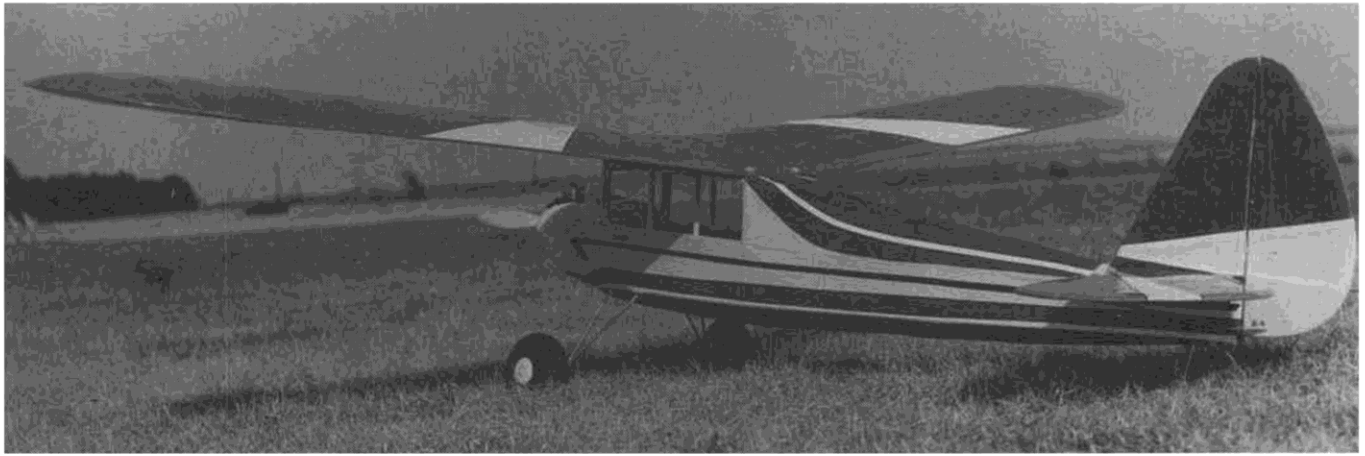
From any angle, "Miss Arpiem" has pleasing lines. Bolt-on wing and stab are not recommended for the novice flyer, and though maybe not as pretty, the good old dowel and rubber bands would be more in keeping with the time of the design, 1938.
