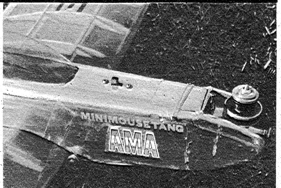
A cozy engine installation. Note the convenient switch location.
